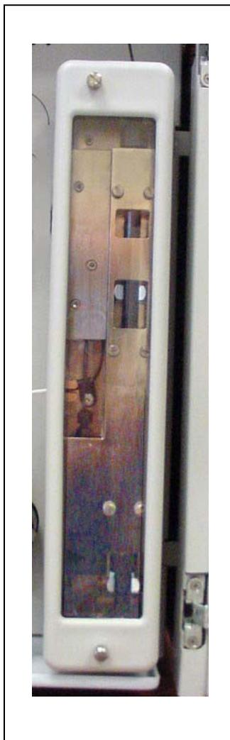
The column heater provides temperature control for the separator and guard column.
