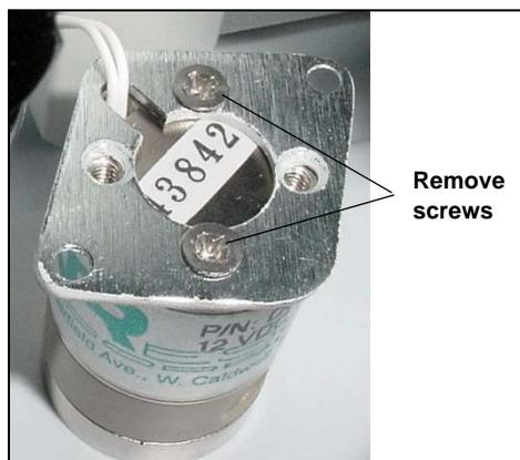
Figure 5-20. Removing the Eluent Valve Mounting Plate
