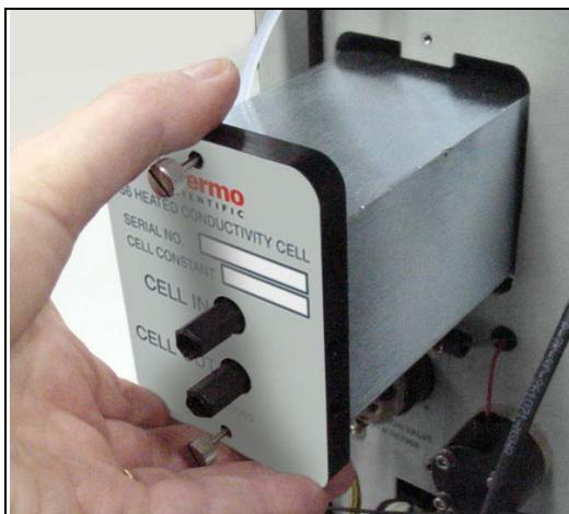
Figure 5-13. Removing the Cell Assembly
