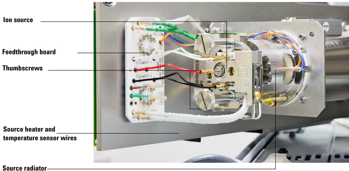
**Figure 11** Removing the standard EI ion source
