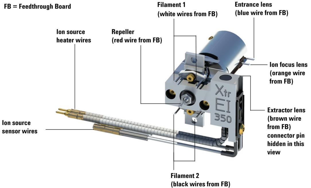
**Figure 21** Ion source wiring - Extraction source shown, standard ion source similar
