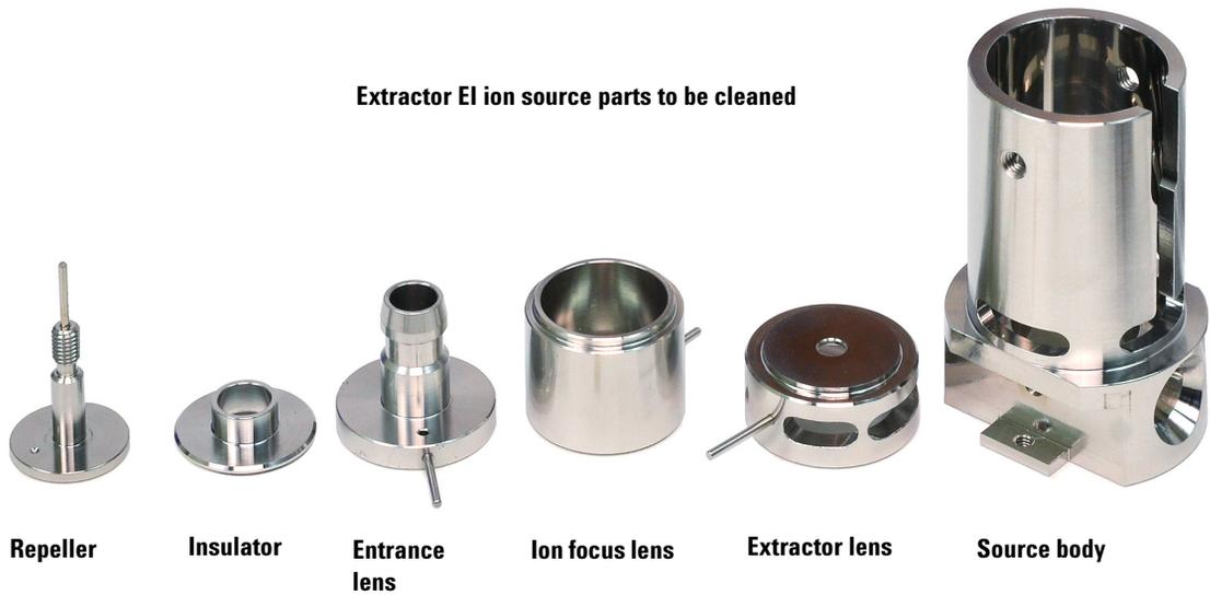
**Figure 15** Source parts to be cleaned
