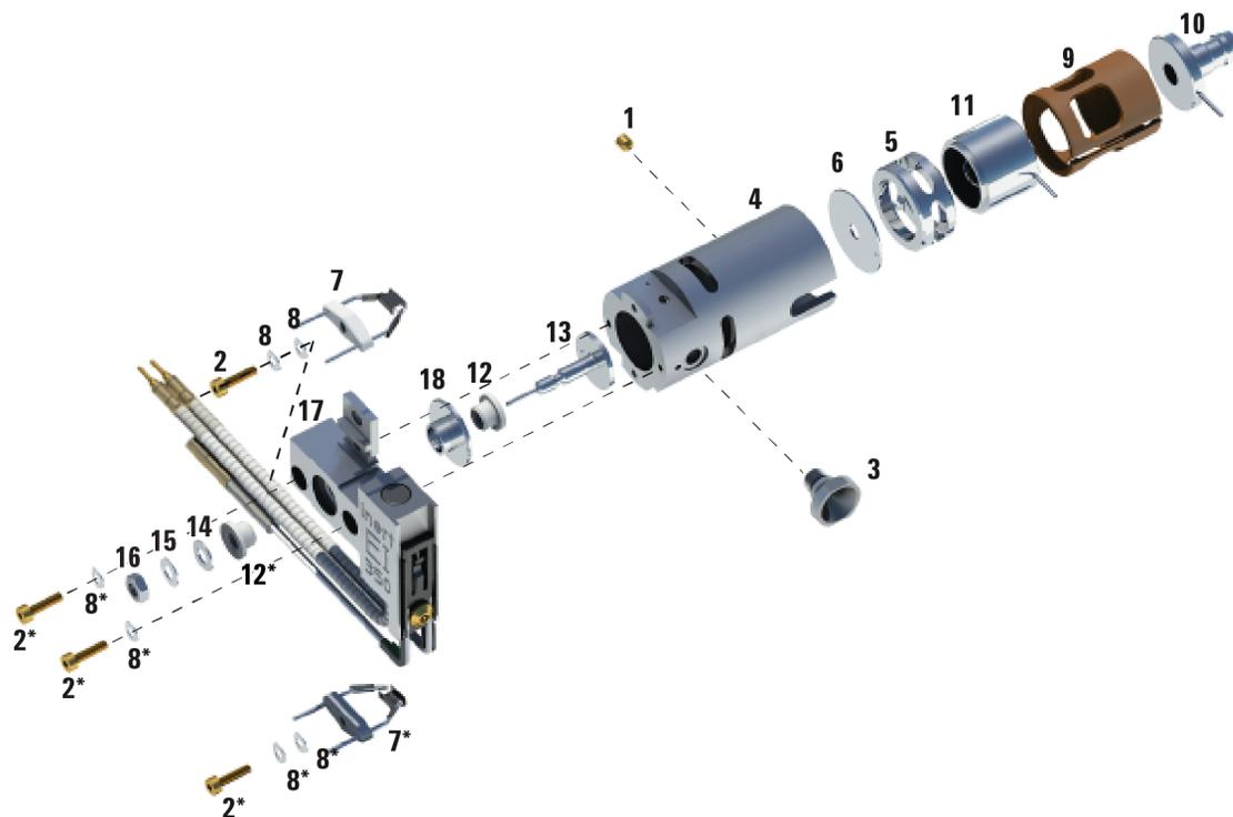
Figure 13 Disassembling the standard or inert EI ion source
