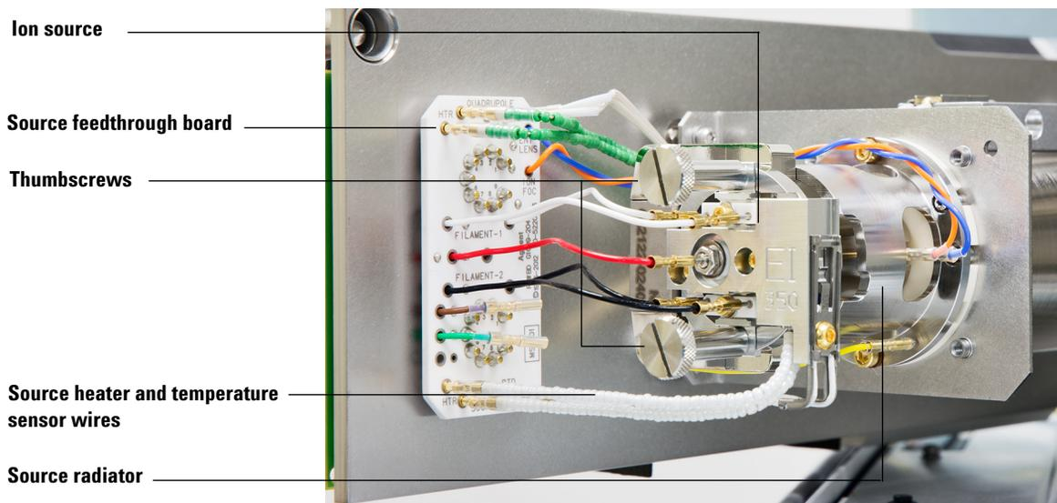
**Figure 19** Installing the EI ion source
