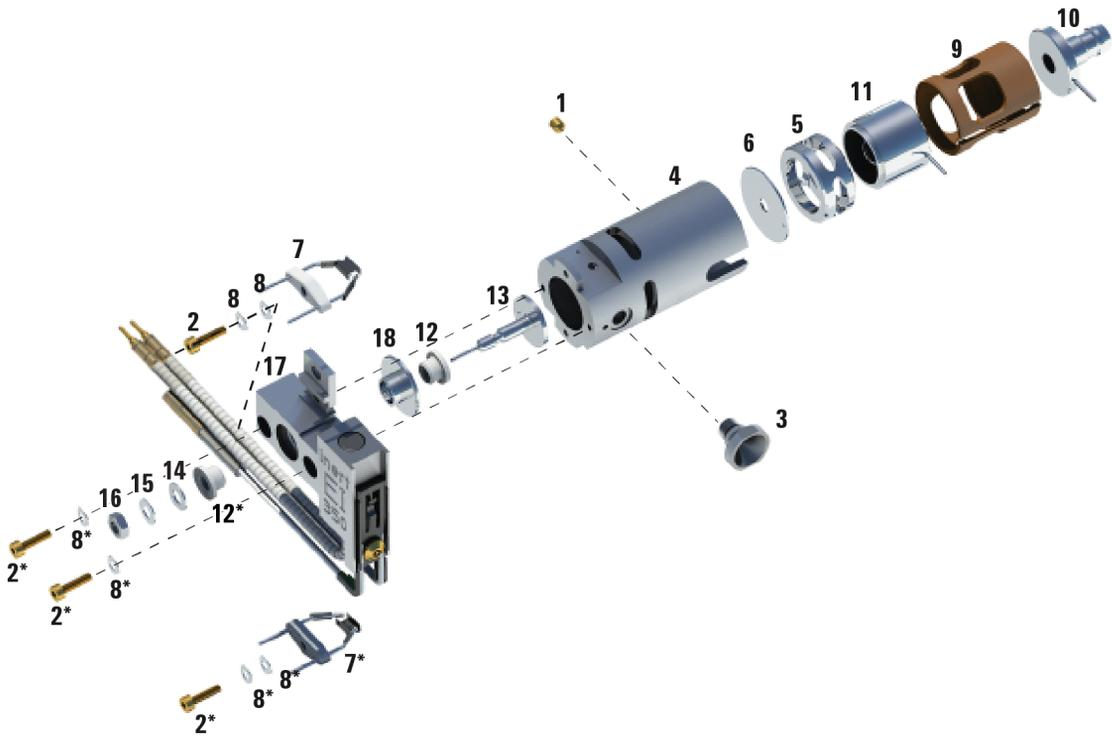
**Figure 16** Assembling the standard or inert EI ion source
