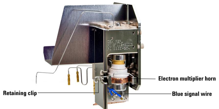
**Figure 22** Replacing the EM horn (Series 2 shown) Series 1 similar
