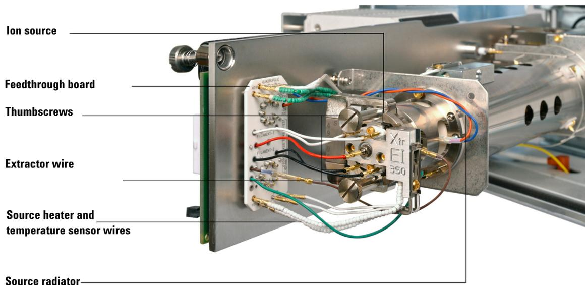
**Figure 12** Removing the Extractor ion source
