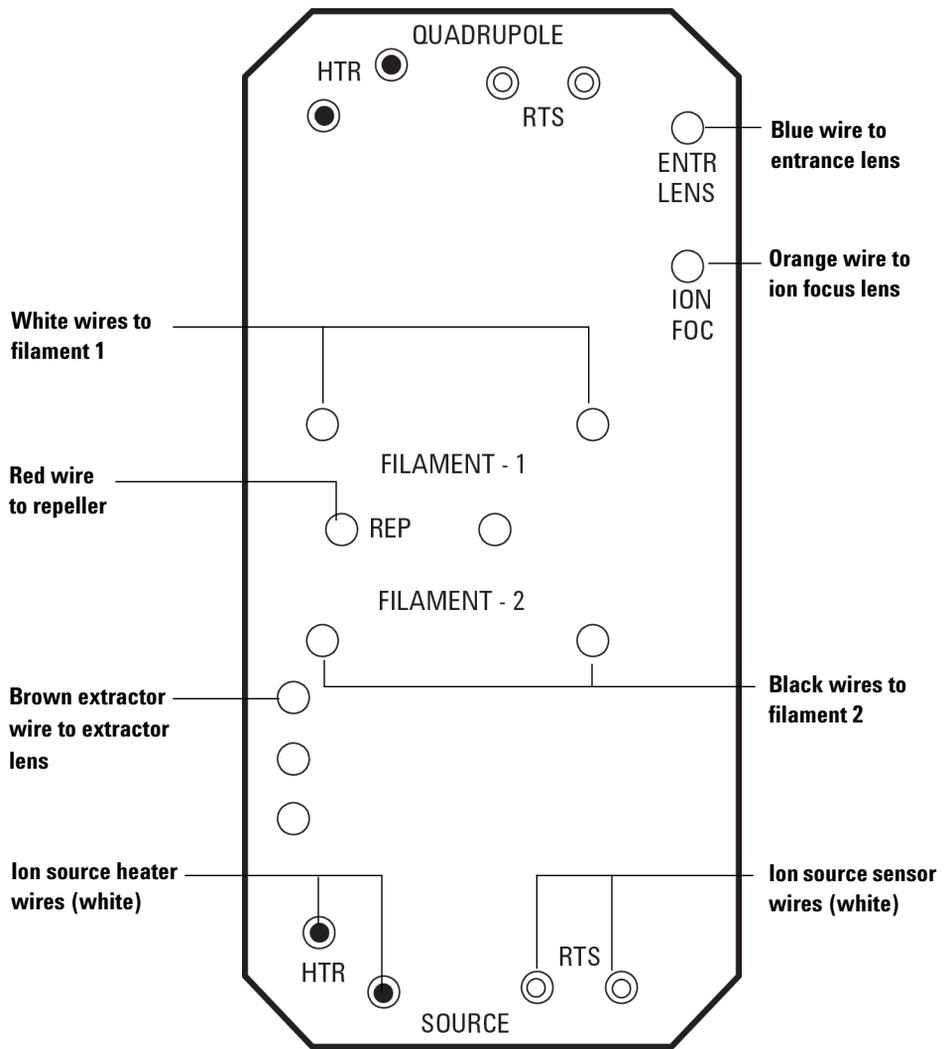
Figure 20 Feedthrough board wiring
