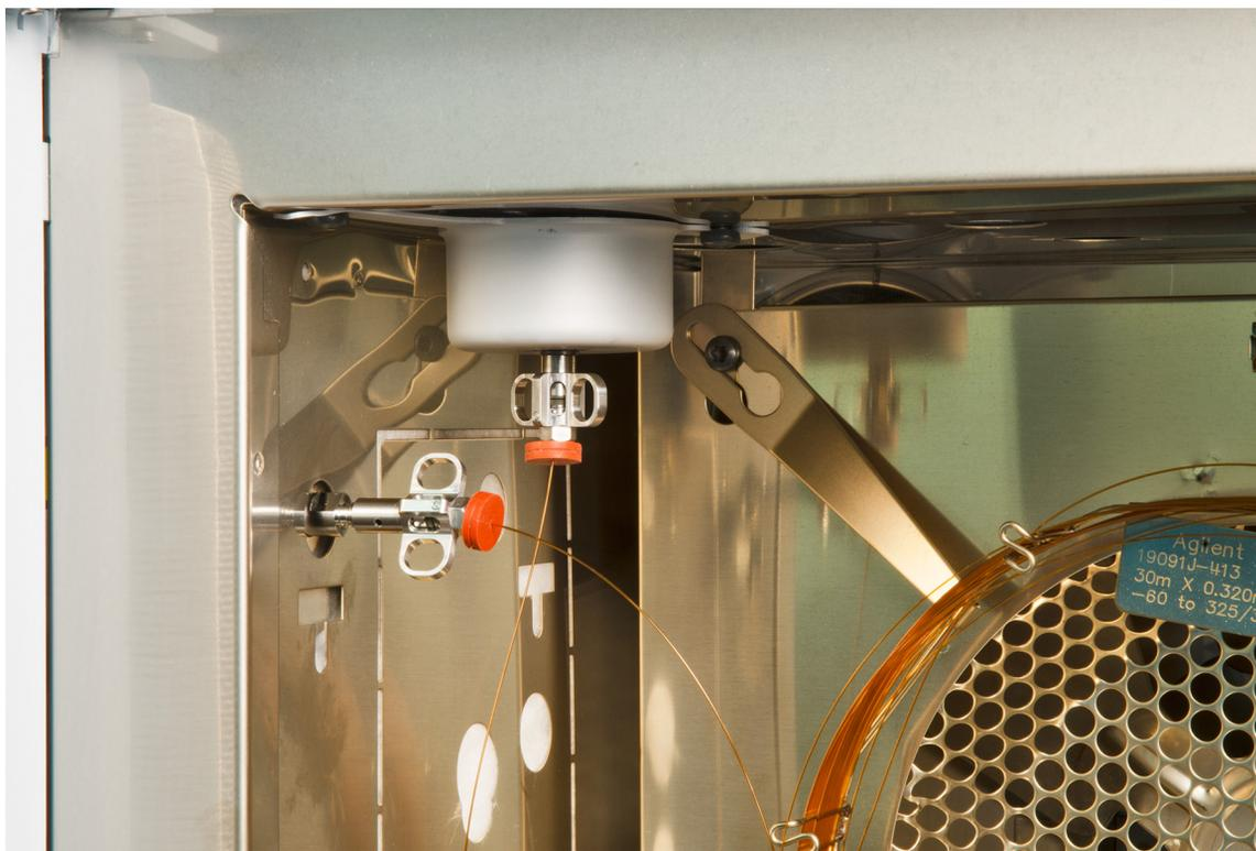
**Figure 6** Installing a capillary column in the GC/MS interface
