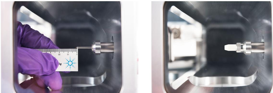
**Figure 5** Installing a capillary column in the GC/MS interface for an EI source.
