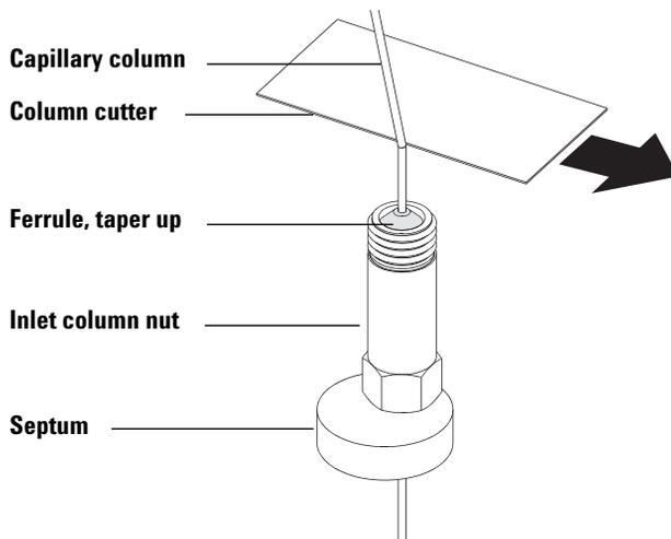
**Figure 3** Preparing a capillary column for installation
