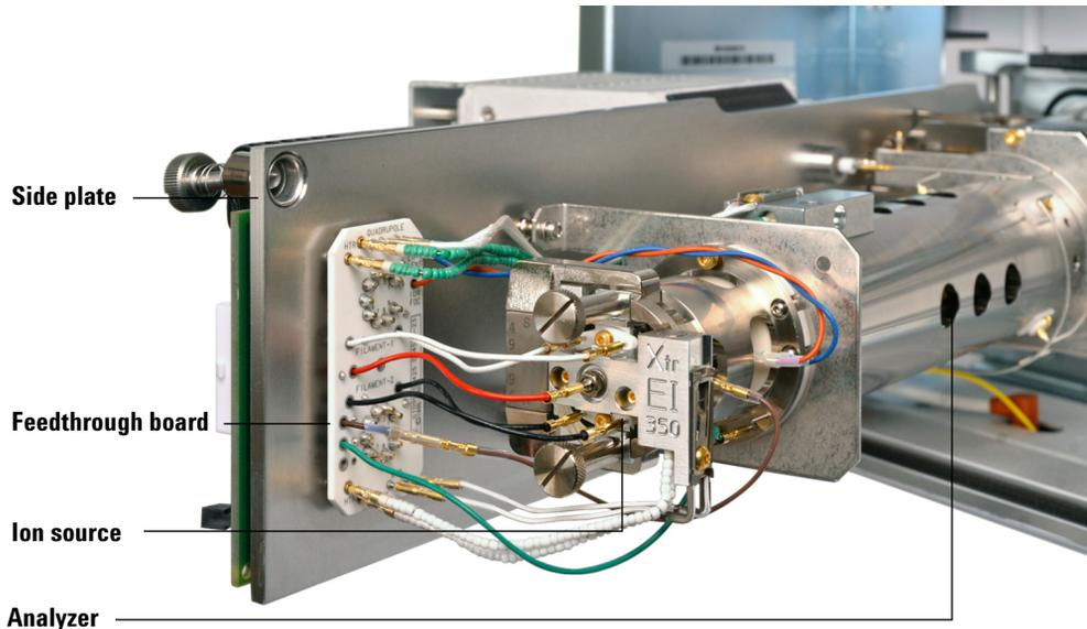
**Figure 10** The analyzer chamber
