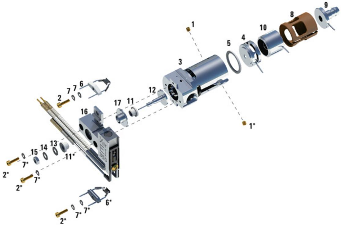
**Figure 14** Disassembling the extractor EI ion source
