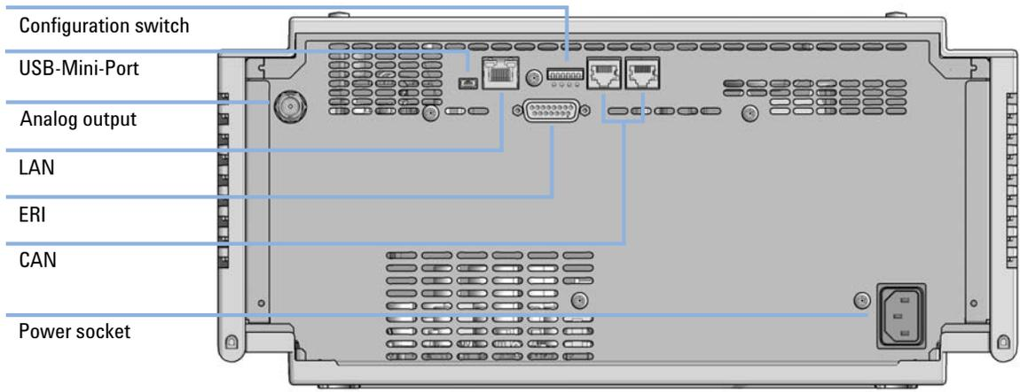
Figure 28 Rear view of the Refractive Index Detector
