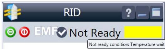
Module Status shows Run / Ready / Error state and "Not Ready text" or "Error text"
