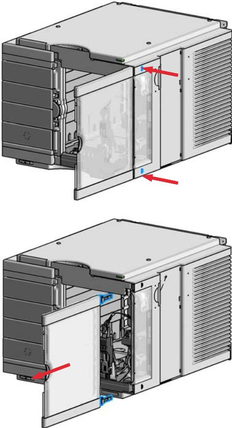
2 For the Installation of the front door. Insert the hinges into their guides and move the door in until the release buttons click into their final position.
