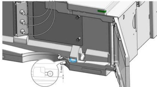
**3** Observe the interface ports for leaks and correct, if required.
