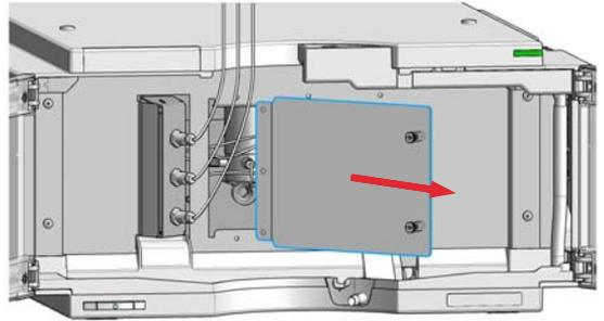
7 Observe the valve area for leaks and correct, if required.
