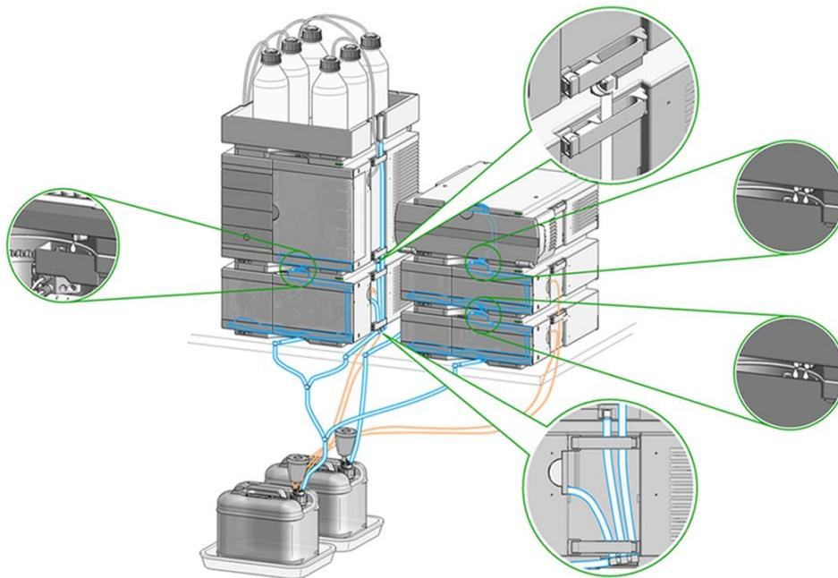
**Figure 12** Infinity II Two Stack Leak Waste Concept (bench installation)
