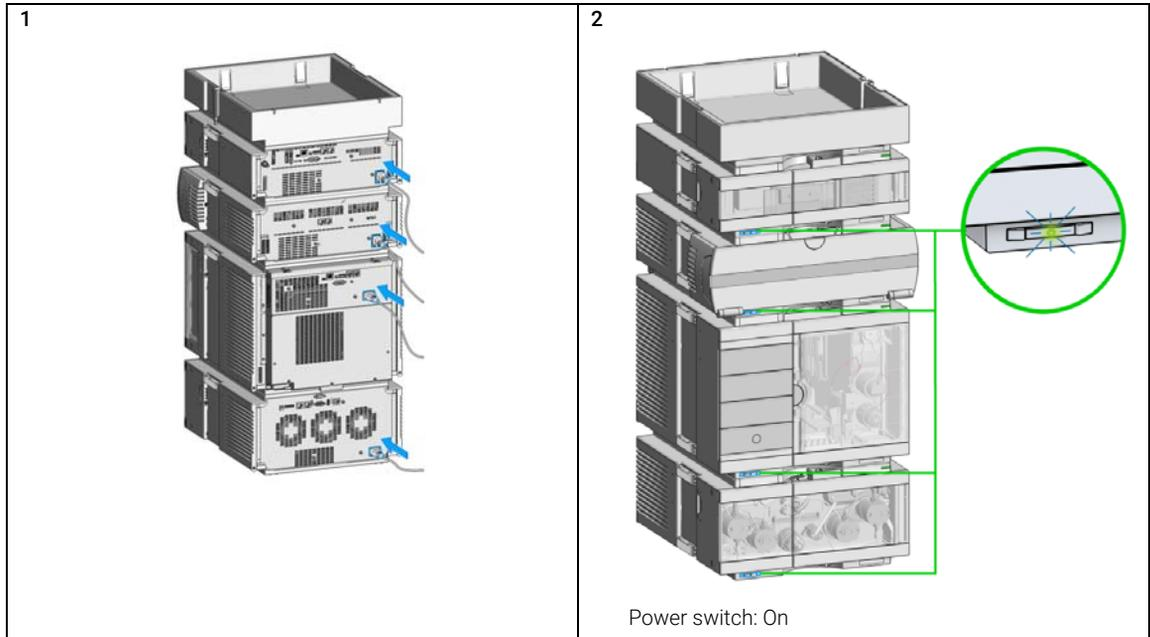
3 Turn instrument **On/Off** with the control software.
