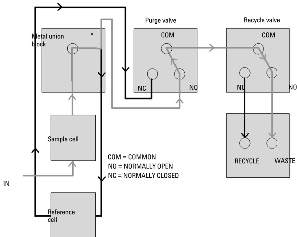
Figure 8 Flow path with the Purge- and Recycle-Valves = OFF
