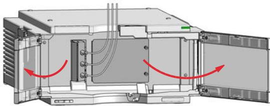
**2** Observe the leak sensor area for leaks and correct, if required.
