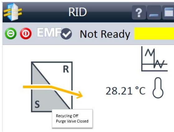
The Purge Valve status (closed/open) and the Recycle Valve status (off/on) is shown when the cursor moves across the flow cell icon.
