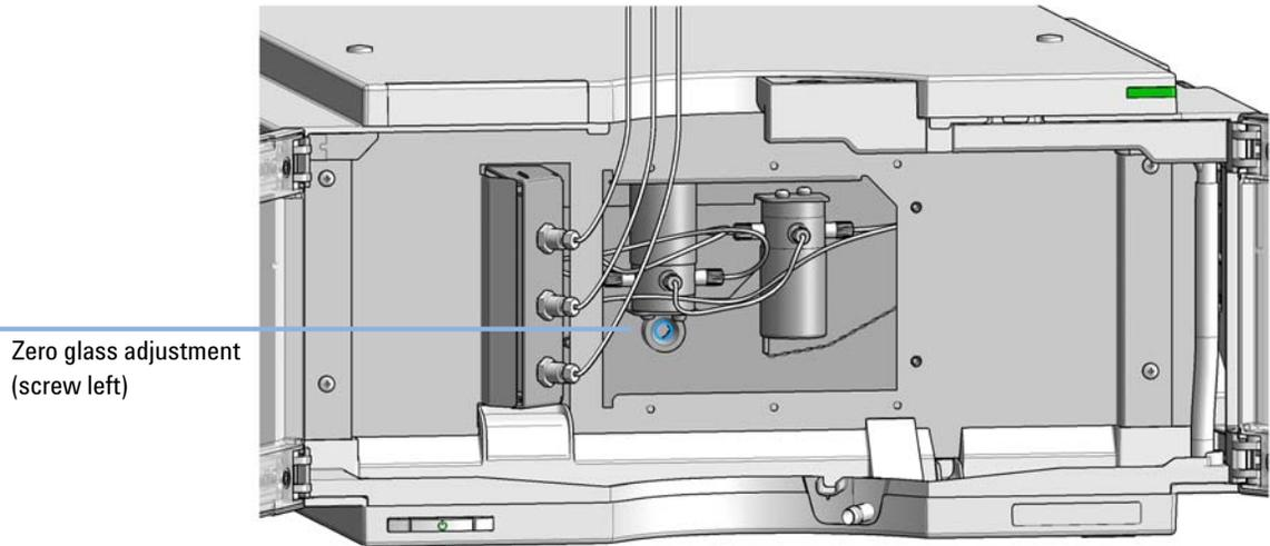
**Figure 21** Turning the zero glass adjustment screw
