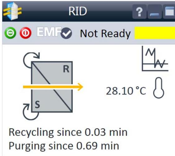
If the Purge Valve or Recycle Valve has been turned on, the on-time is displayed below the flow cell icon.
