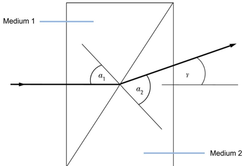
Figure 4 Light Refraction
