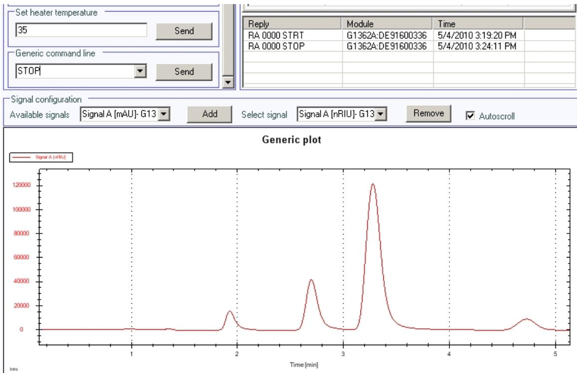
Figure 22 Test Chromatogram with Agilent Lab Advisor
