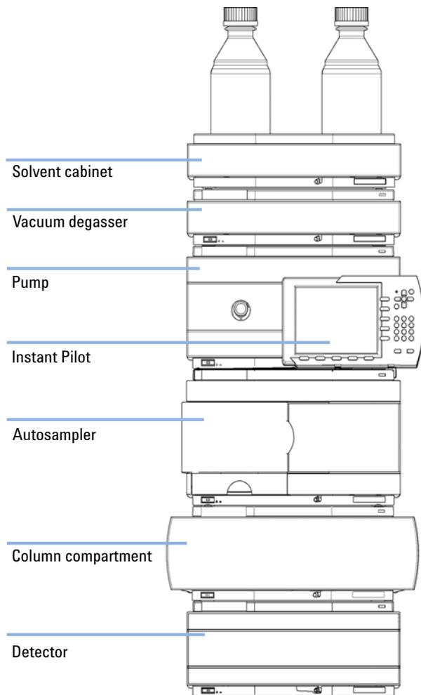
**Figure 7** Recommended Stack Configuration for 1260 Infinity (Front View)
