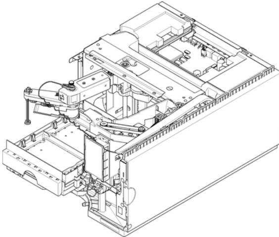
**4** Flip the Leak guide open.
