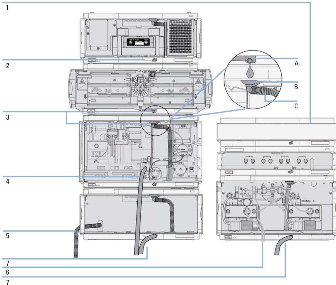
**Figure 6** Leak and waste handling concept (overview - typical stack configuration as an example)
