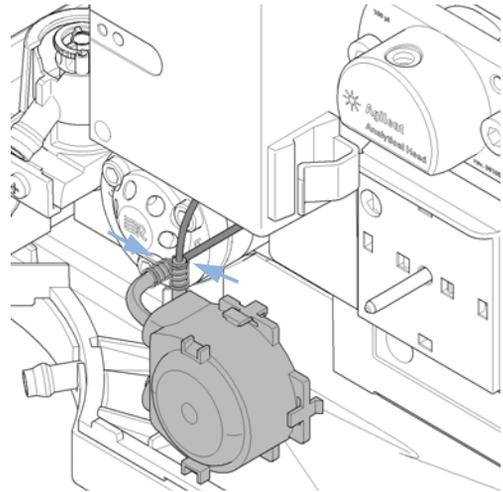
**5** Connect the wash port tubing to the upper tubing of the new cartridge (use sand paper to get a good grip on the tubing).
