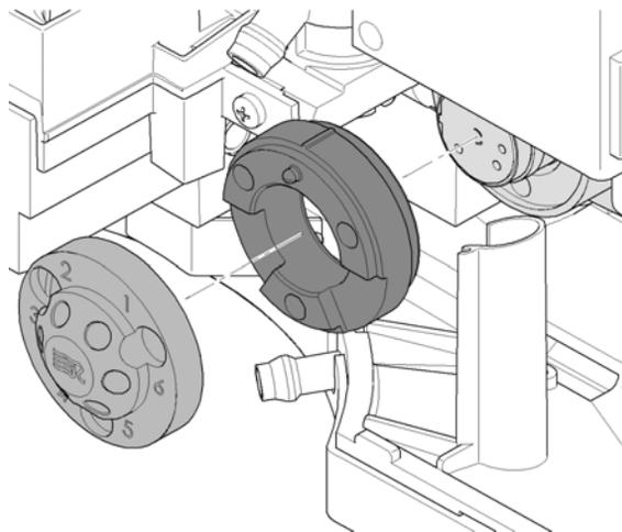
**9** Insert and tighten the stator screws alternating with the 9/64 inch hex key, until the stator head is secure.
