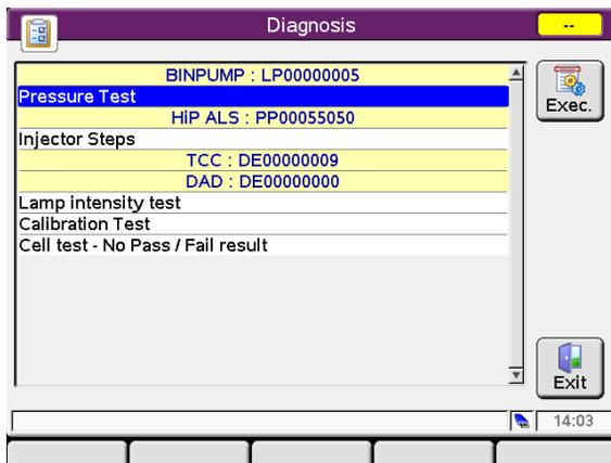
The **Diagnosis** screen provides access to module specific tests.
