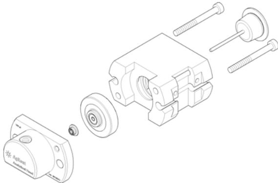
**8** Carefully remove the metering seal using the steel side of the insert tool. Clean the chamber and ensure all particulate matter is removed.
