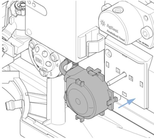
**8** Reinstall the corrugated leak tubing.
