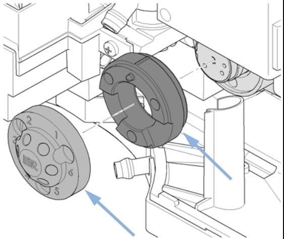
**5** Remove the rotor seal.
