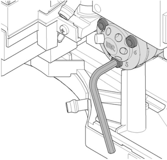
**4** Remove the stator head and the stator ring.
