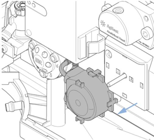
**4** Disconnect the tubing leading to the wash port and the tubing coming from the solvent bottle.
