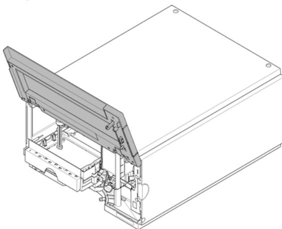
**3** Disconnect the seat capillary from the Injection valve.
