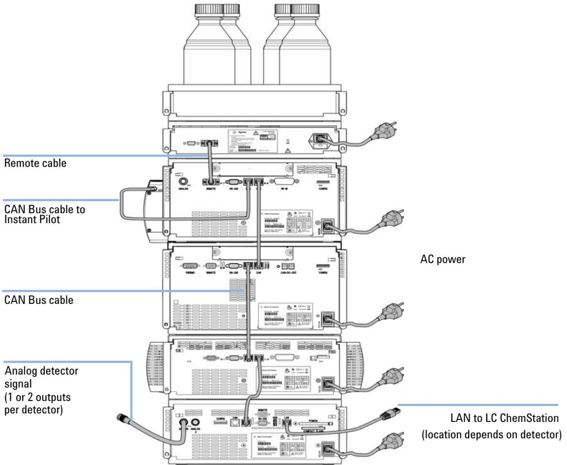
**Figure 8** Recommended Stack Configuration for 1260 Infinity (Rear View)
