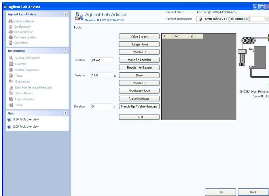
**Figure 28** Injector Steps—Running
