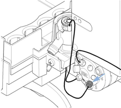
**4** With a Flat head screw driver carefully lift out the needle seat from the holder.
