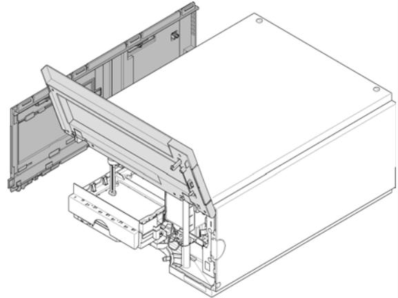
**3** Turn the Needle carrier 90 ° clockwise.
