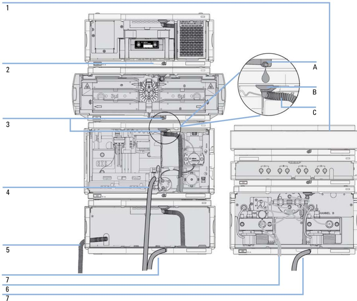
**Figure 11** Leak and waste handling (overview - typical stack configuration as an example)
