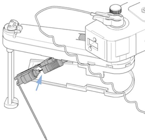
**3** Pinch the holder clamp and reinsert the needle assembly into the needle carrier.
