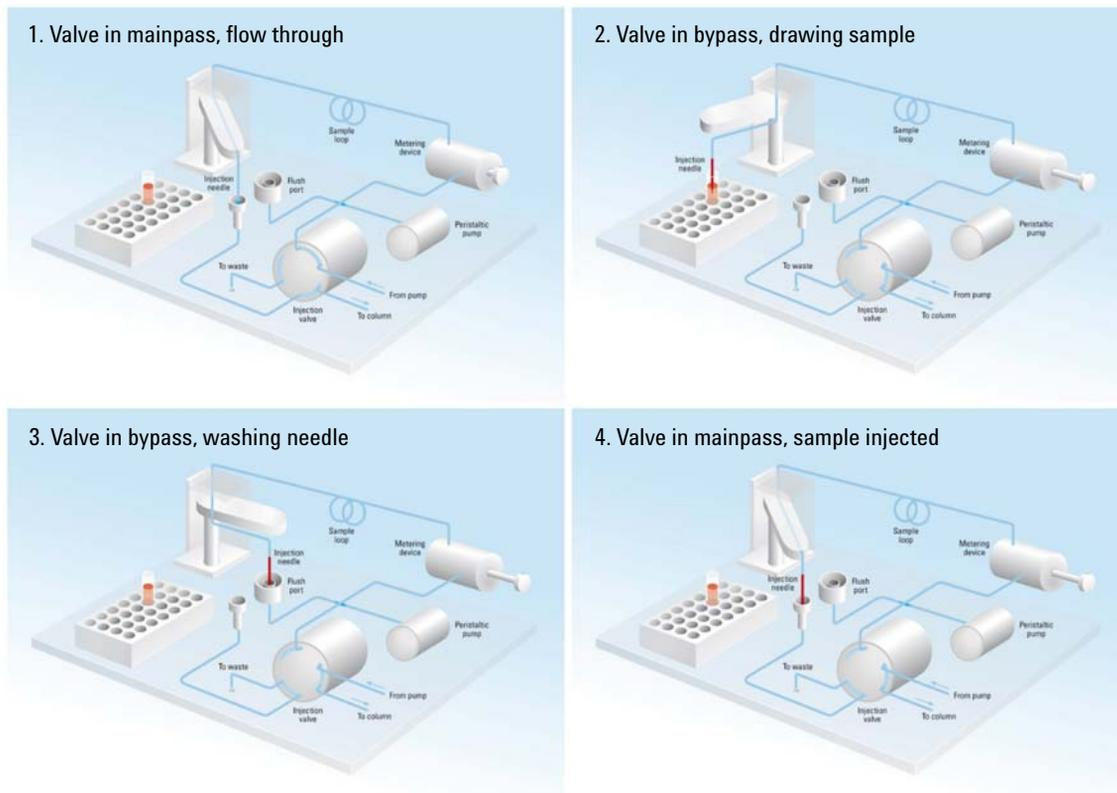
**Figure 16** Schematic of injection steps in 1260 Infinity Autosampler
