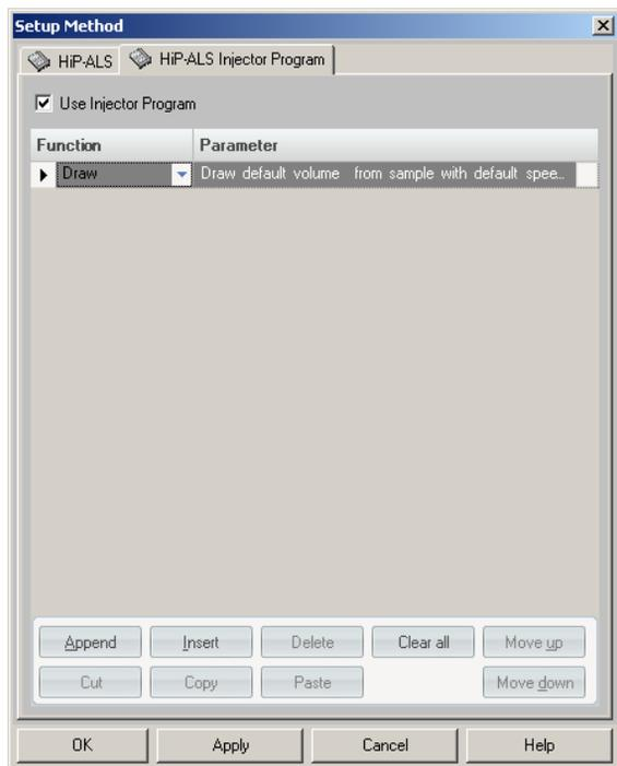
The pretreatment/injector program comprises a series of numbered lines, each specifying an operation that the autosampler carries out sequentially. When you activate a pretreatment/injector program, it replaces the standard injection cycle.
