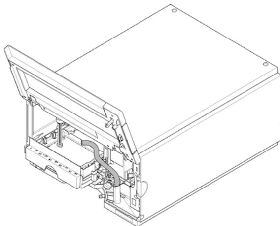
**2** Press the two clips on the front of the peristaltic pump cartridge.
