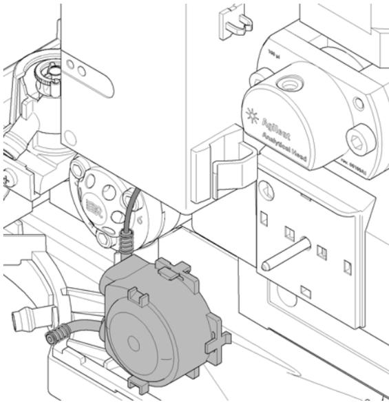
**6** Connect the tubing coming from the solvent bottle to the lower tubing of the new cartridge.
