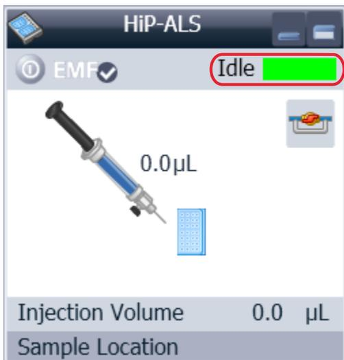
**Module Status** shows Run / Ready / Error state and “Not Ready text” or “Error text”.
