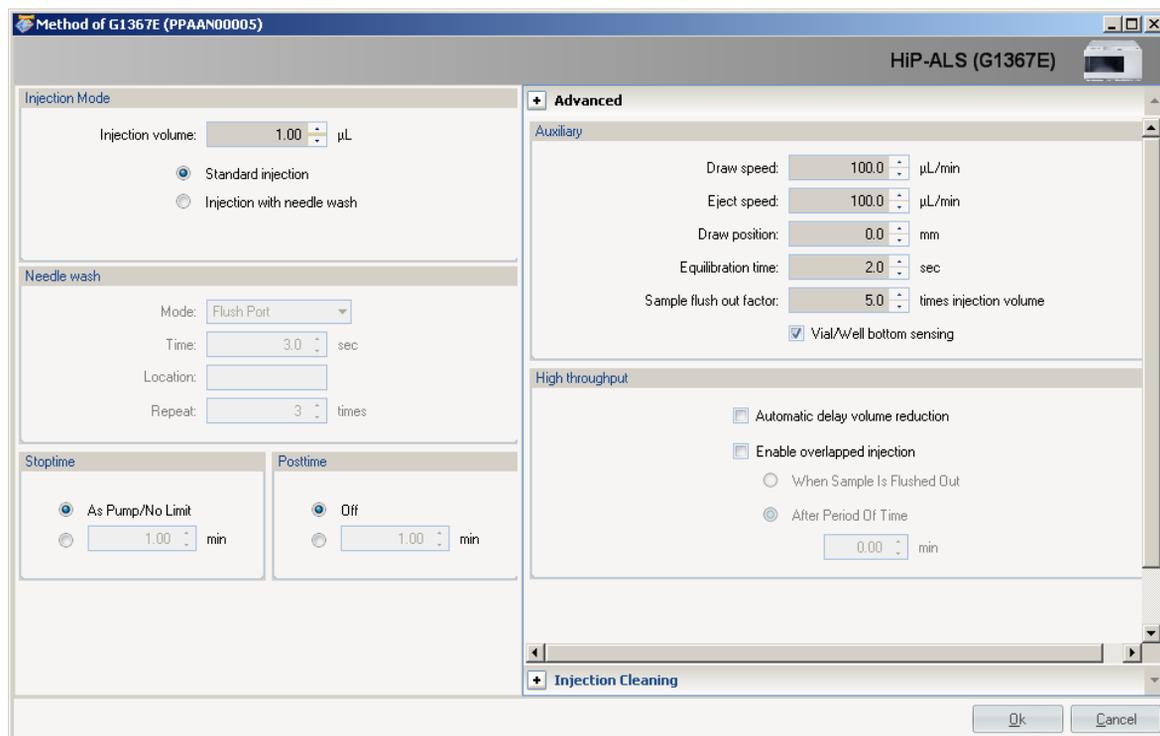
**Figure 15** Method Parameter Settings
