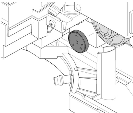
**8** Reinstall the stator ring and stator head. The pins on stator ring and stator head must engage in the corresponding holes.
