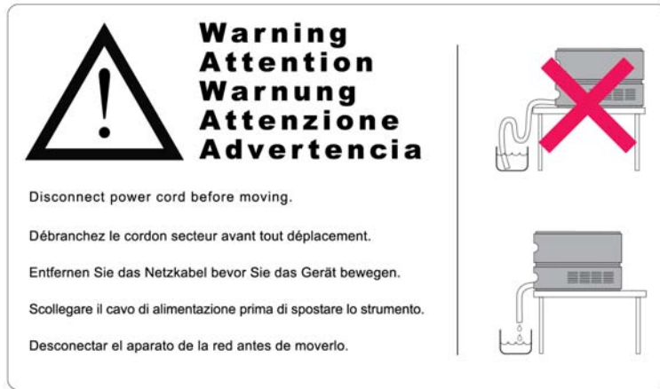
Figure 23 Warning label (illustration for correct waste tubing)
