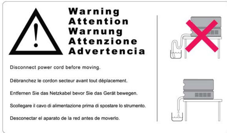
Figure 13 Warning label (illustration for correct waste tubing)
