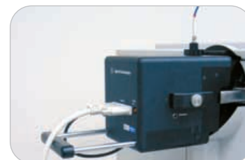
Pulsed Dynamic Focusing MALDI (PDF-MALDI) Source
