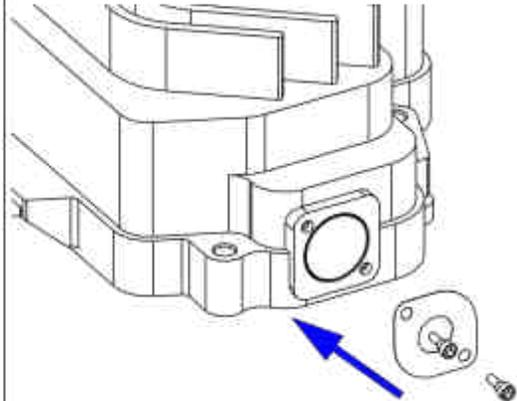
8 Replace the lamp housing cover and fix the screws. Carefully insert the rear foam. Reconnect the monochromator cables to the main board. Left is excitation, right is emission.
