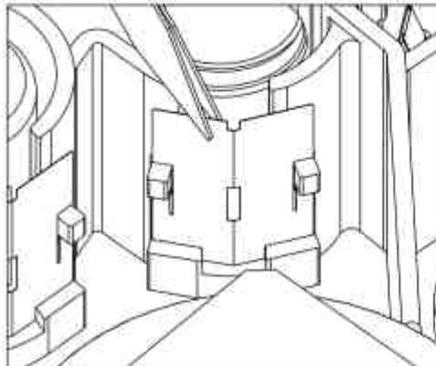
**5** Put slight pressure on to the spring part of the slit.
