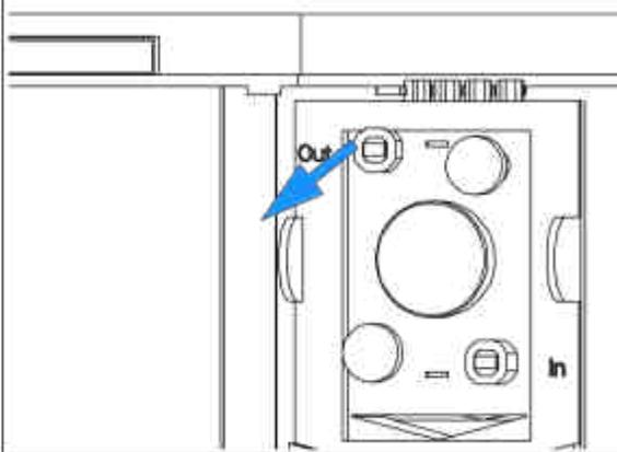
**3** Assemble the column detector capillary from the accessory kit. One side is already factory-assembled.
