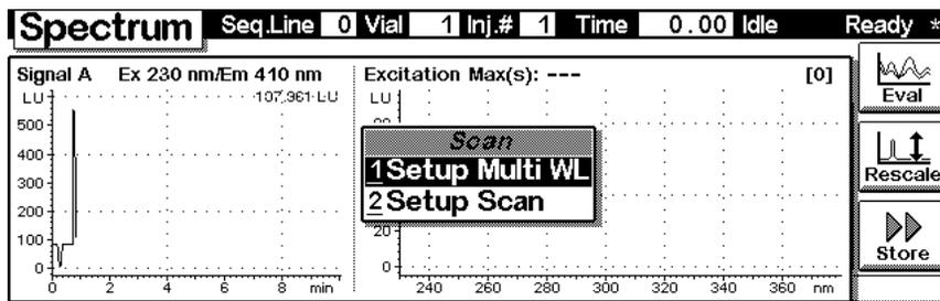
From Menu item 1 (**Setup Multi WL**) you can switch between Excitation and Emission spectra and choose simultaneous multi-wavelengths detection.
