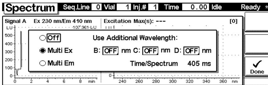
From Menu item 2 (**Setup Scan**) you can set spectra acquisition parameter. Store spectra is only valid if an Agilent Chemstation is connected.
