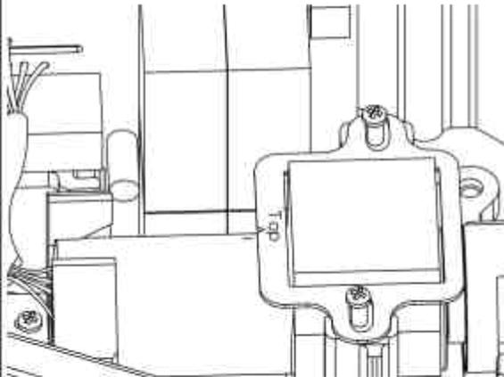
**12** While pressing the top pad down onto the stand-offs, tighten the screws. Turn the trigger pack such as its marker stays in line with the "TOP" sign of the brass holder.
