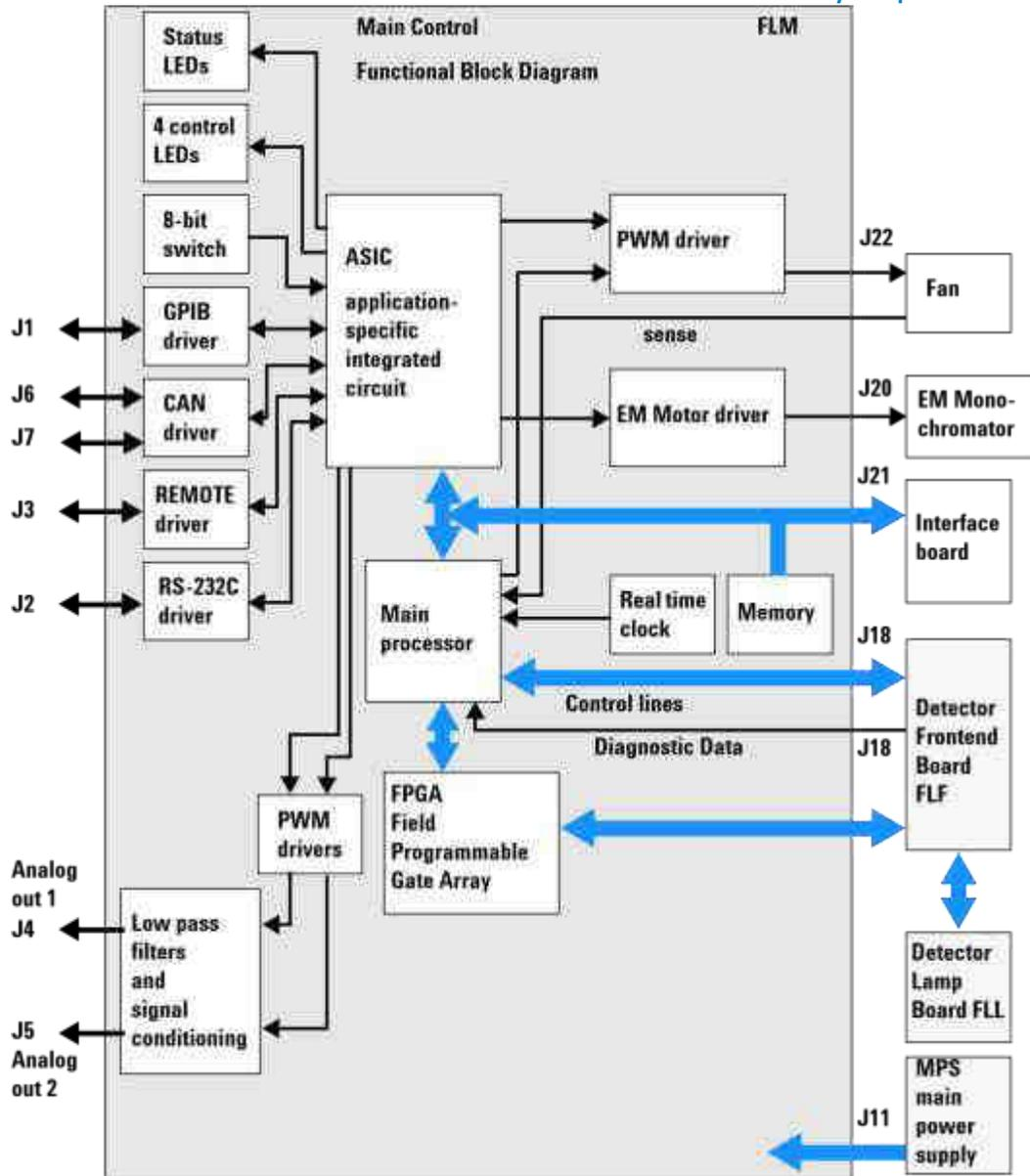
**Figure 88** Block Diagram FLD Main Controller Functionality
