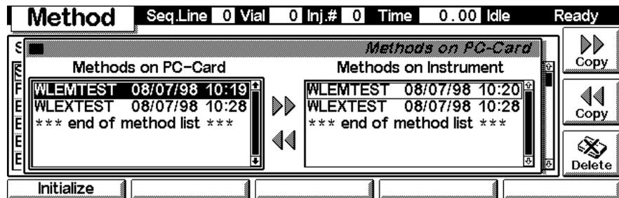
**Figure 36** Copying Methods into the FLD
