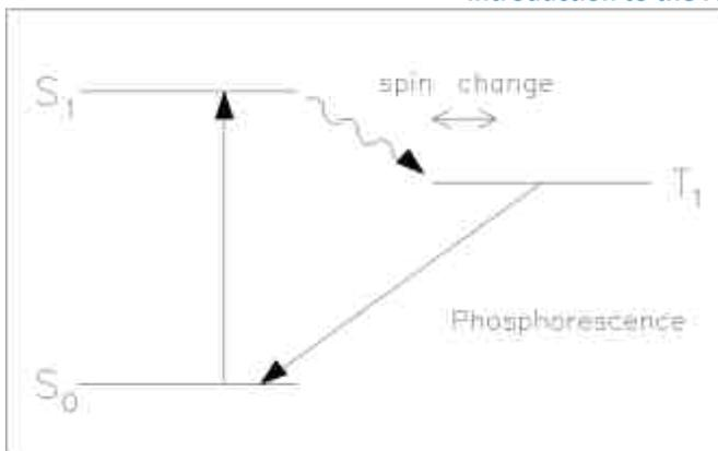
**Figure 72** Phosphorescence Energy Transitions
