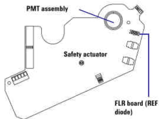
**5** If you need to replace either the board or the PMT assembly, remove the PMT assembly from its socket.
