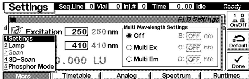
Selecting **More** and **Settings** pull down menu you can enter special FLD setpoints. The **PMT-Test** allows the automatic check for optimum signal/noise and dynamic range under current conditions in the flow cell.
