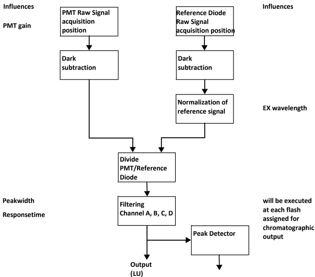
**Figure 93** Data flow for chromatographic output
