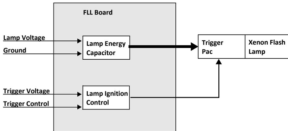
**Figure 90** Block Diagram FLL Board
