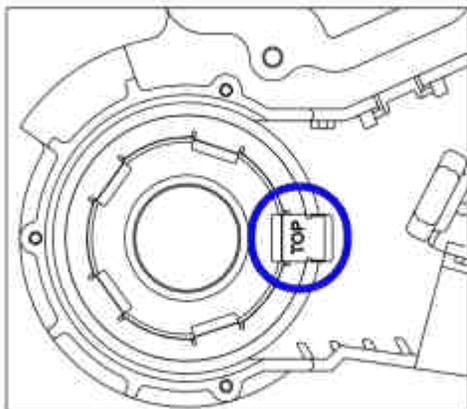
**5** For reinstallation route the cable first through the hole. Carefully insert the grating into its position while pulling the cable slightly from below. The couple spring has to be clipped into the protection ring (TOP mark)!
