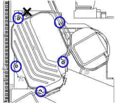
4 Using the 2.5 mm hexagonal key, unscrew one screw and loosen the other one. Slide the window holder out of the window area.
