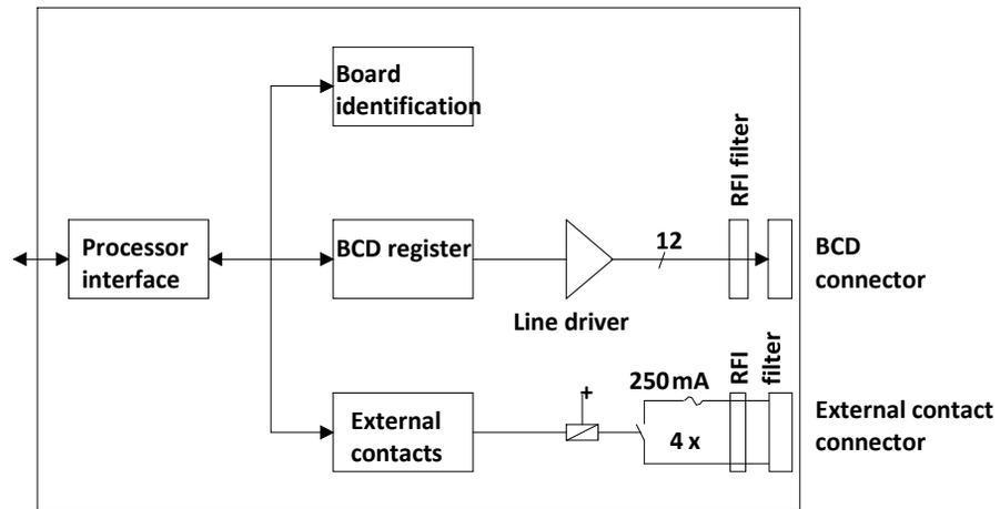
**Figure 95** Block Diagram BCD Board
