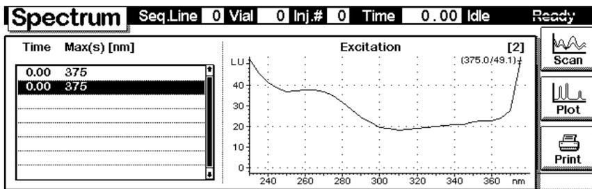
During spectra review press the **m**-key to open the context sensitive menu. The menu item 1 (Clear All Spectra) empties the memory in the Control Module. The menu item 4 (Save Spectrum) leads to the next screen.
