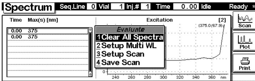
With a PC card inserted into the Control Module spectra can be stored as \*.csv files and viewed with Microsoft Excel “ software. Letters of the filename can be entered by pressing several times the numerical keys (see *Reference Manual of the Control Module*).
