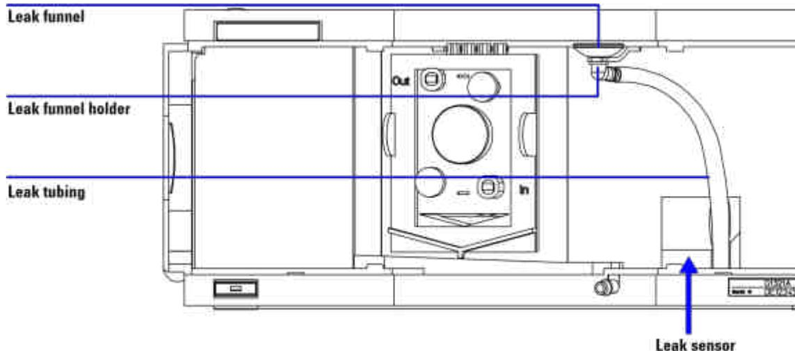
Figure 54 Replacing Leak Handling System Parts
