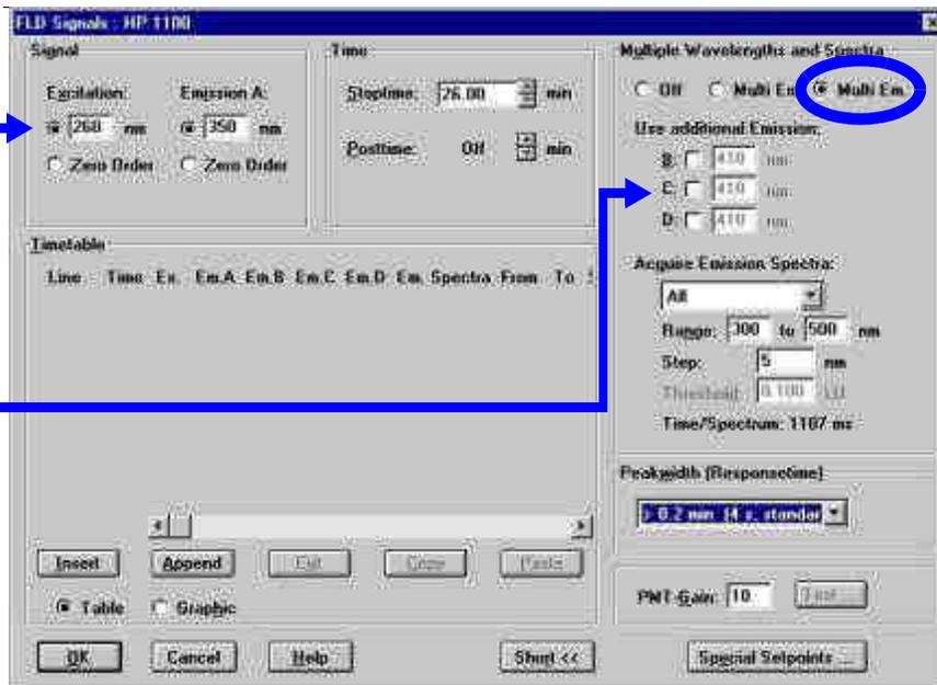
**Figure 18** Detector Settings for Emission Scan
