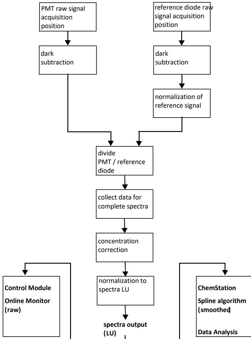
**Figure 94** Data flow for spectral output
