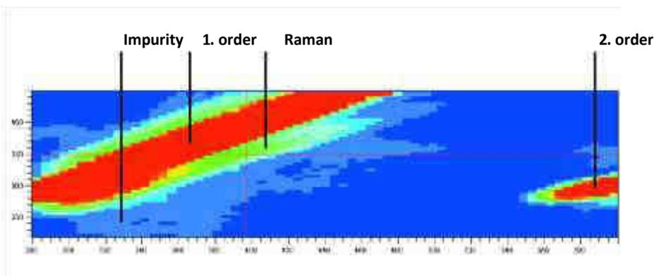
**Figure 10** Isofluorescence plot of a mobile phase
