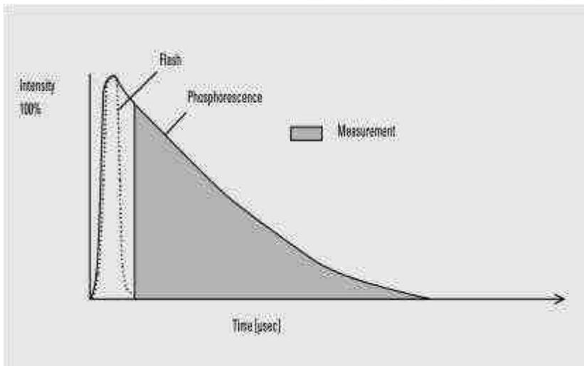
**Figure 81** Measurement of Phosphorescence
