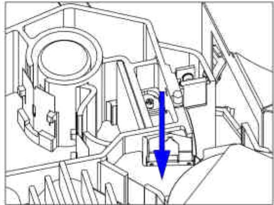
**If the mirror is inserted in the opposite direction, the detector cannot be aligned correctly.**
