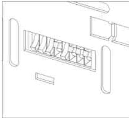
**Figure 97** 8- bit Configuration Switch
