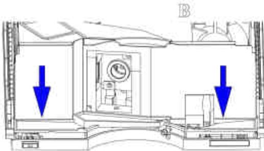
8 Replace the leak sensor using your left hand and reconnect the connector.
