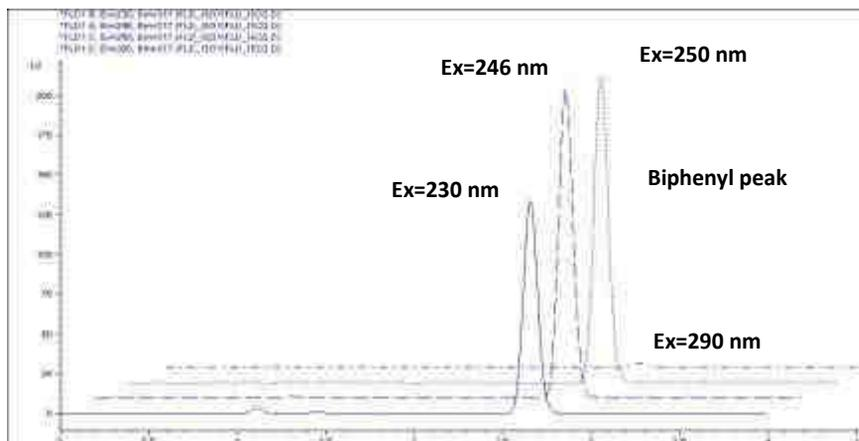
Figure 8 Biphenyl peak with different excitation wavelengths
