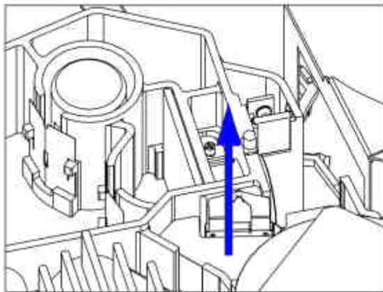
**3** Locate the three slits (from left to right: PMT, EM, EX).
