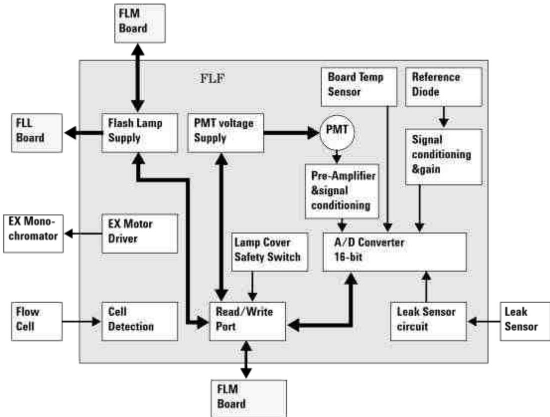
**Figure 89** Block diagram FLF Reference System
