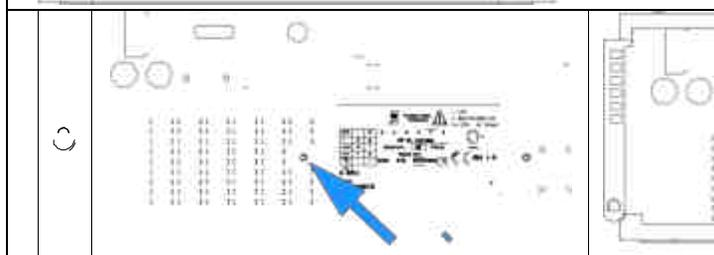
**3** Press down the power switch light pipe to remove it from the coupler.
