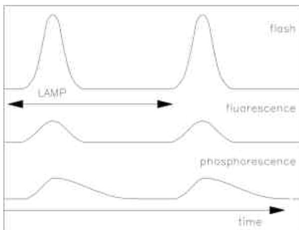
**Figure 82** LAMP: Frequency of Flash, Fluorescence, and Phosphorescence
