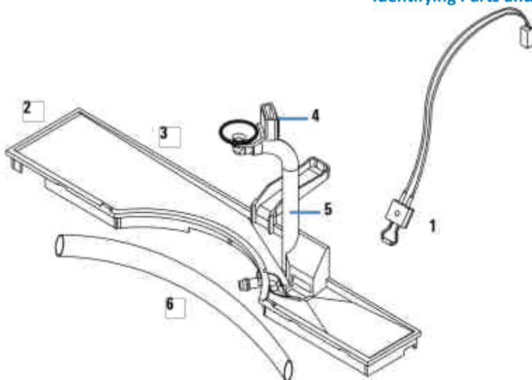
Figure 66 Leak Parts
