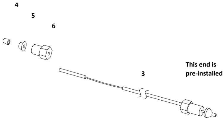
Figure 68 Inlet Capillary (Column-Detector) Parts
