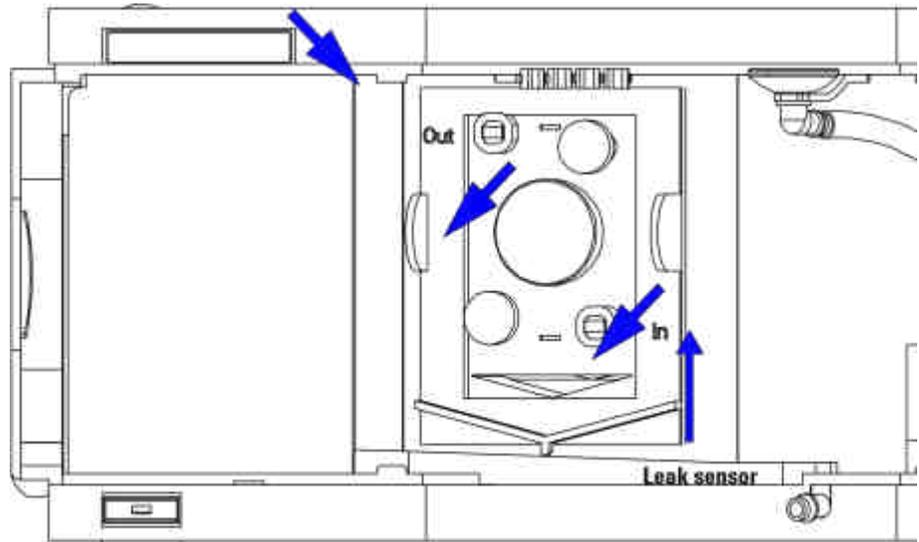
**Figure 53** Observing for Leaks
