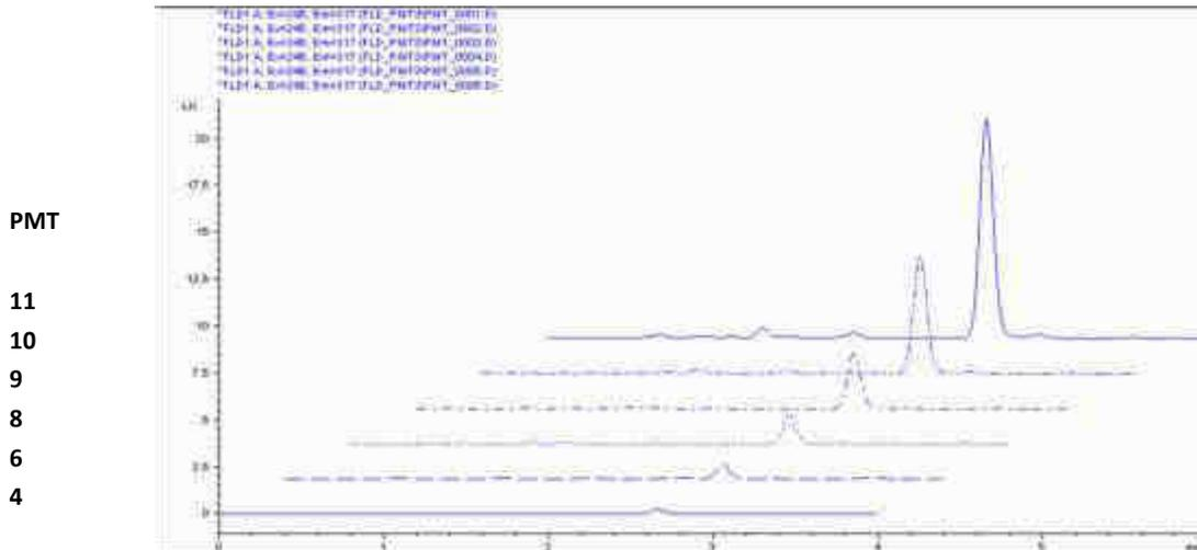
**Figure 27** Finding Best PMTGAIN for Biphenyl
