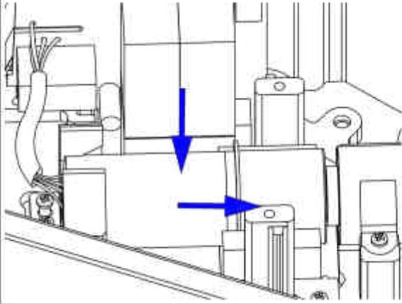
**10** Refit the trigger pack holder by moving the lamp towards the condenser. Leave a distance of about 0.5 mm between each other. Refit the screws.
