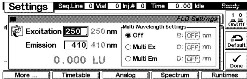
Use the **m**-key for the context sensitive menu. The **Status** command pulls up a monitor screen displaying signals and spectra as programmed. **Reset** will load the FLD default parameters.
