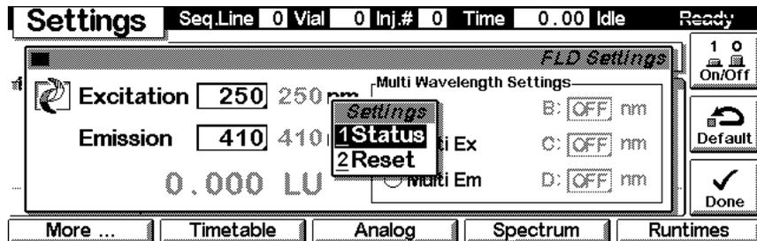
Use F1-key (**More**) opens a pull-down menu. The item **Scan** is available when Multi-Ex or Multi-Em mode has been selected. The **Phosphor** mode is not available with FLD firmware revisions A.03.6X and below.
