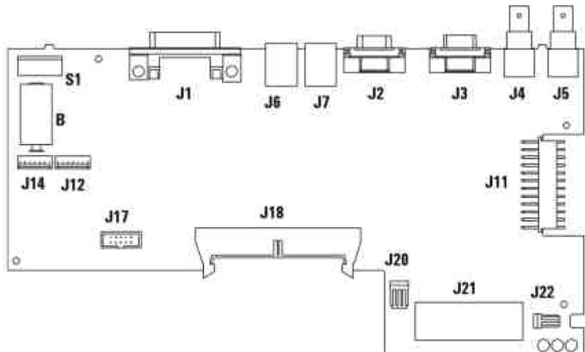
Figure 56 Location of Connectors on FLM Board
