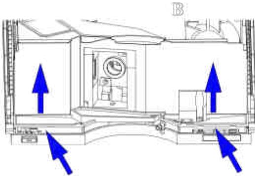
6 Remove the leak base completely.
