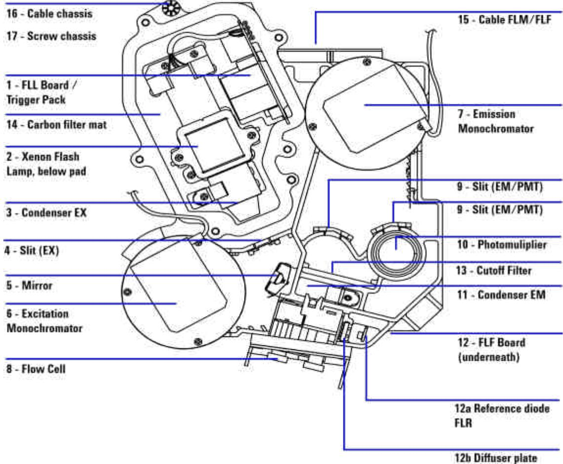
Figure 59 Optical Unit Parts
