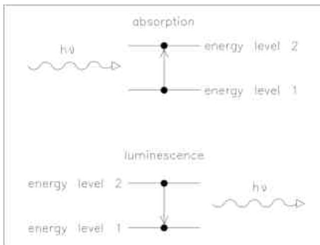
**Figure 70** Absorption of Light Versus Emission of Light
