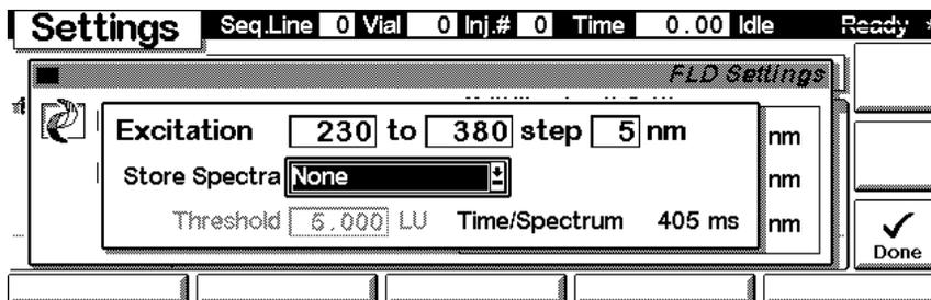
Selecting **More** and **3D-scan** on the pull down menu you can enter setpoints for taking for the 3D-fluorescence scans. Data can only be displayed using the 3 D-Agilent ChemStation software.
