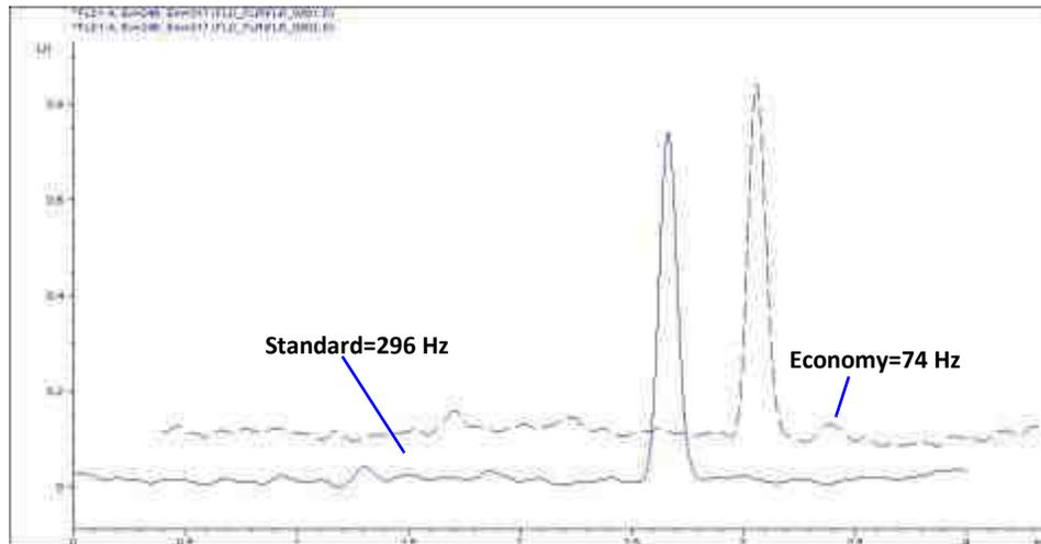
**Figure 28** Xenon Flash Lamp Frequency
