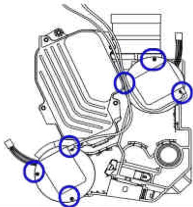
**3** Carefully remove the grating assembly and the protection ring from its location.
