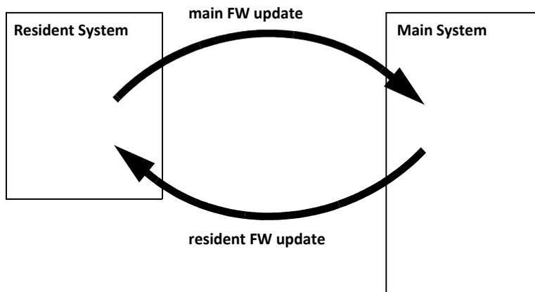
**Figure 91** Firmware Update Mechanism
