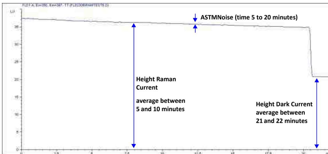
**Figure 48** Raman ASTM signal/noise calculation
