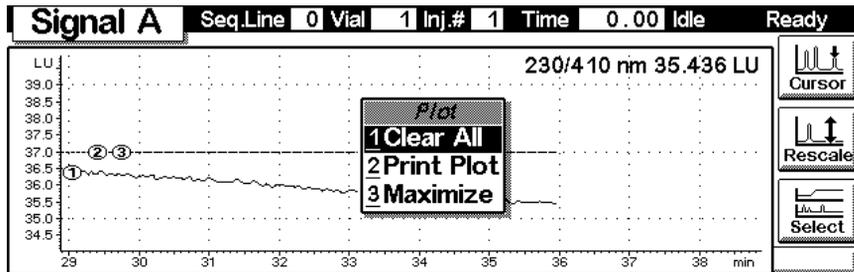
Press F6 key (**Select**). Here you can add additional on-line signals (maximum are 3). Additional signals could be also pressure or temperature signals from other modules. Use the Right/Left arrows to switch between Available and Selected Signals. Use the F8 key (**Move**) to enter available signals into the box for selected signals or vice versa.
