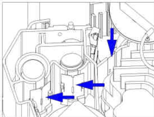
**4** Use a pair of tweezers to replace the slit.
