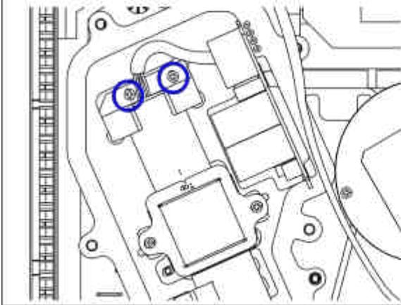
6 Tip the holder to release the lamp and trigger pack. Slide the cables of the trigger pack through the holder.
