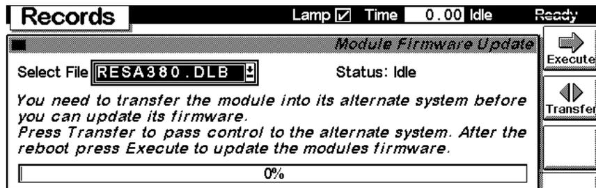
Use the Esc key to receive **Views** on the F5 key. Choose **System** from the pull-down menu. Use the F3 key (**Records**) to select the FLD. Use the F5 key (**FW Update**) to enter the Update section. Select the a file from the PCMCIA card (1321nnnn.DLB) and
