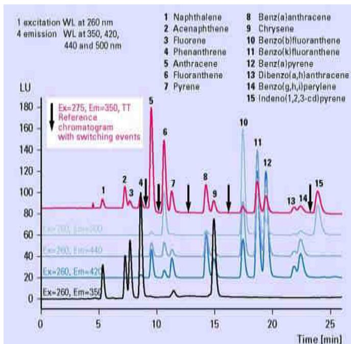
**Figure 17** Simultaneous multi wavelength detection for PNA-analysis
