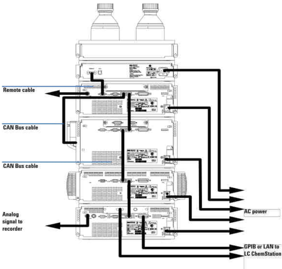
Figure 4 Recommended Stack Configuration (Rear View)
