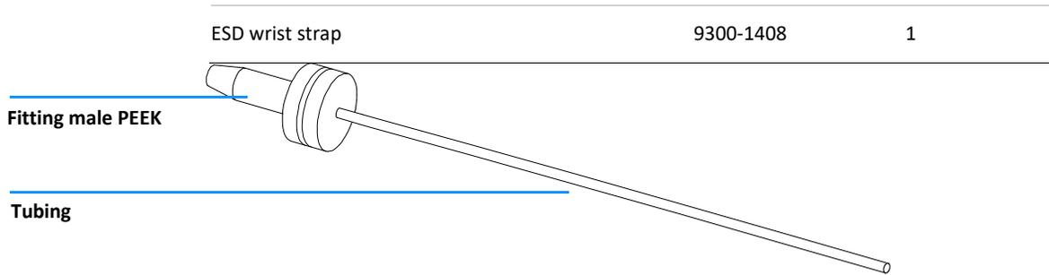
Figure 1 Waste Tubing Parts
