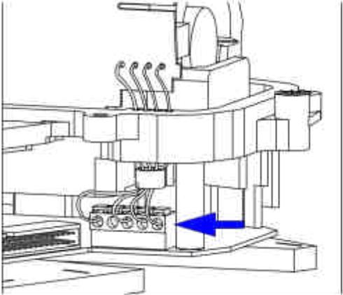
**11** Put the wires into the released contacts using the tweezers.
