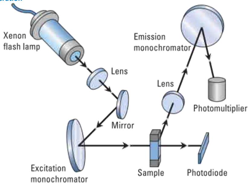
Figure 92 Optical Diagram of the FLD
