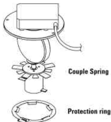
**4** Insert the new protection ring into its position. Do not bend the protection ring.
