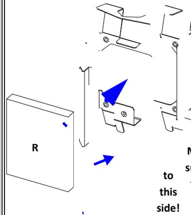
8 Replace the mirror assembly and lock the top over the pin.
