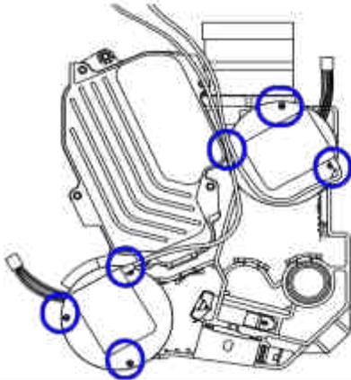
**7** Assure the UV protector cover is installed. Replace the foam on the optical unit.
