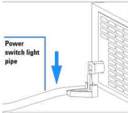
**4** Remove the power supply completely. Re-use the coupler on the new power supply.
