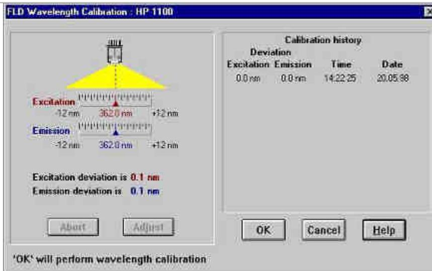
Figure 41 Wavelength Calibration - User Interface
