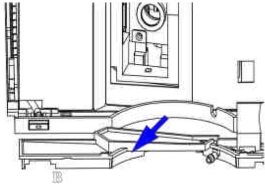
7 Replace the leak pan into the cabinet bottom. Press the leak pan completely down into its recess.
